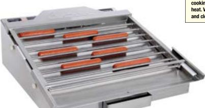
The Cretors patented stainless-steel hot dog grill design includes a center drive shaft that reduces the number of moving parts from six to two, ensuring longer motor life and allowing full rotation of the product on the grill. The stainless-steel cooking surface has an aluminum heat plate underneath that evenly distributes heat. Visual digital temperature controls allow for precise temperature setting, and clear visual temperature display.
